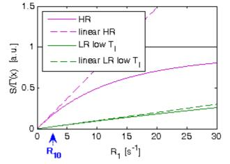
**Fig 1.** Signal curves for both SR-TurboFLASH protocols considered in the text: the LR centric-reordered, low-TI protocol can be well approximated by a linear curve, while the HR linearly ordered higher-TI protocol cannot.
