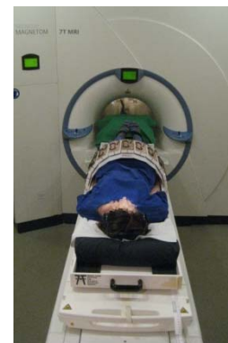
Figure 1: Examinations were performed with a manually positionable AngioSURF table. The custom-built 16-channel coil was positioned surrounding the table with 5 elements beneath and 11 elements above.
