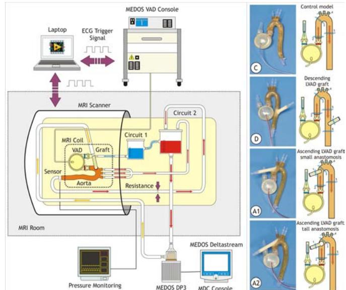
Fig. 1: Illustration of the model system to investigate different outflow cannula positions as illustrated in the right panel. The MR compatible VAD inside the scanner simulates the failing heart; the “true” VAD is positioned outside the scanner due to its non-MR compatibility (MEDOS DP3). In the right panel placed emitter planes for flow quantification are shown.
