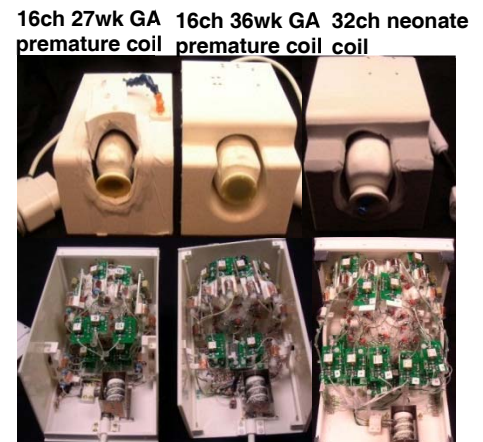
Fig. 1: Arrays with 3D-printed plastic head phantoms (top); elements laid out on formers (bottom).
