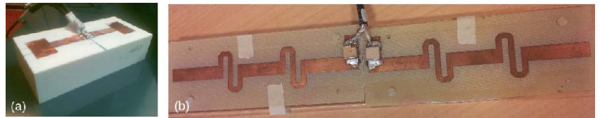
Figure 2: a) Single-side adapted dipole antenna (SiSiAD) b) Fractionated dipole antenna (FD)
