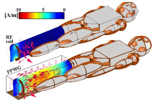
Fig. 2. Poynting vector simulations: top) RF coil only and b) RF coil plus PPWG.
