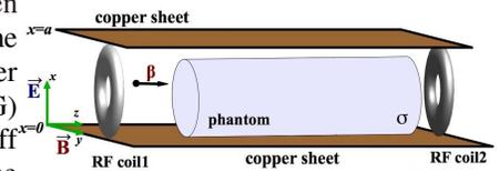
Figure 1. PPWG simulation setup of B1.
