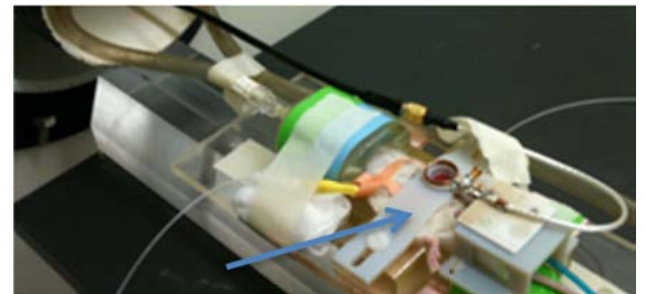
Fig. 2. Animal support structure. Plastic part (arrow) clamps the WC in place. Surface coil is mounted over the WC.
