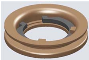
Fig. 1. WC structure with coverslip retaining ring.
