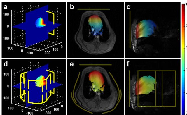
**Fig. 1:** Magnetic field simulation for the single surface coil (a, b and c) and the 5-channel array coil (d, e and f). a and d are the 3D field distribution. b and e are the field distribution overlaid to an axial anatomical image of a pig heart. Similarly c and f are the sagittal field distribution.
