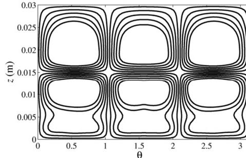
Fig.1: First-order irregular shim array (one quadrant).
