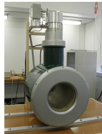
Figure 1: 1.5 T Cryogen Free MRI. The magnet bore has a 260 mm ID and the outer dimensions are 550 mm OD, 1030 mm tall and 535 mm long.
