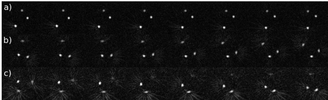
Figure 2: 8 frames taken from 3 time series with the rotational frequency set to a) 0.5Hz, b) 1Hz and c) 1.5Hz. The frames show a time series of 160ms. Streaking artifacts intensify with increasing rotary frequency. Rotation is counter-clockwise, time elapses from left to right and images are windowed accordingly.
