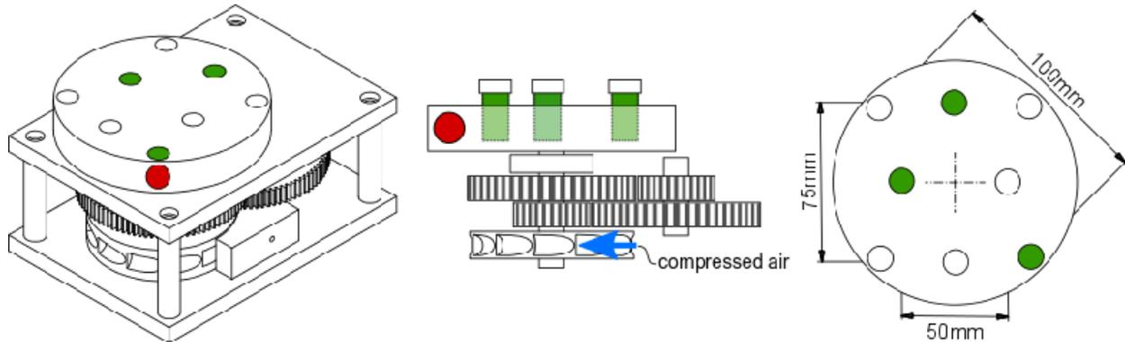
Figure 1: Mechanical drawing of motion phantom showing slotted rotor, gear wheels (ratio 1:9), rotating disc and positions of test-tubes.
