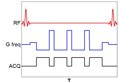
Fig. 1: The present sequence acquires four separate pairs of FISP (S<sup>+</sup>) and PSIF (S<sup>-</sup>) signals during a TR of about 21 ms. As usual in a DESS-like sequence, the G<sub>freq</sub> pre-phaser is 1/4th the area of the readout.
