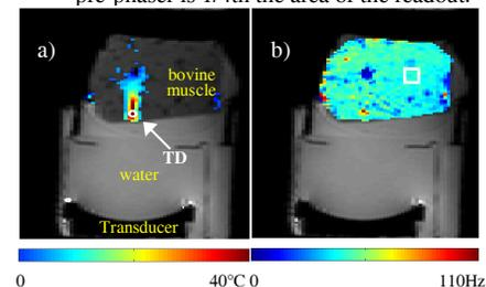
Fig. 2: Temperature (a) and R<sub>2</sub> (b) map for the time frame with peak temperature. See text for details.
