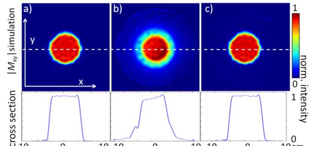
Fig.2: Bloch simulations of  $M_{xy}$  for segmented excitation a) without, and b) with 800Hz off-resonance, c) with corrected off-resonance.
