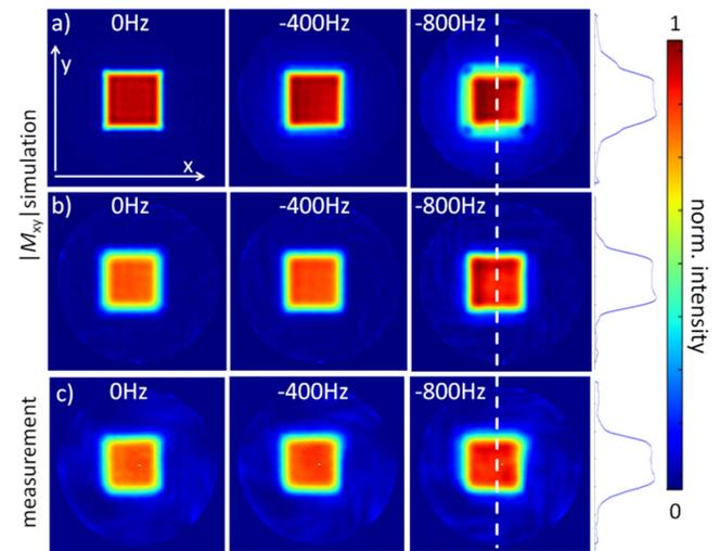
Fig.3: off-resonance performance of segmented SSE for a) standard calculation, b) & c) off-resonance optimized pulse
