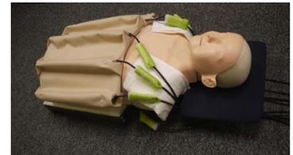
Fig 1: Transmit-array coil used.
