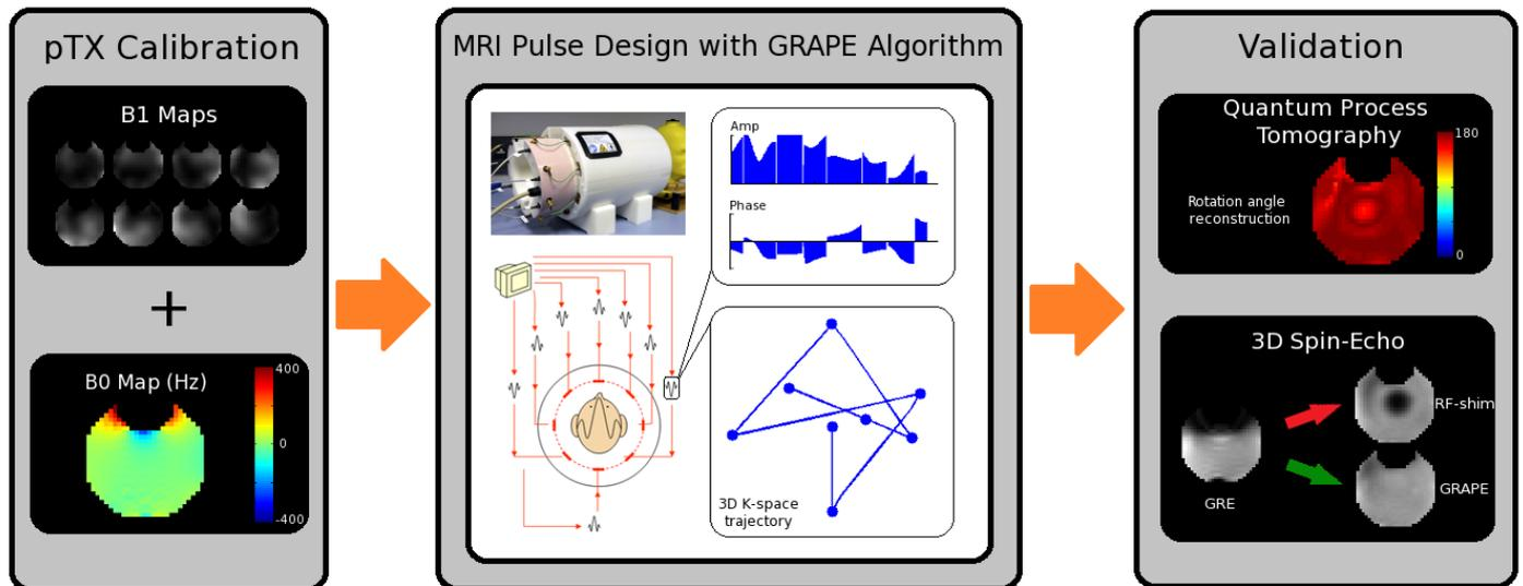
**Figure:** Step1: pTX Calibration. Step2: Optimization Process. Step3: Experimental Validation (Top: Quantum Process Tomography results: rotation angle. Bottom: Phantom signal with: Excitation only (GRE), modified Spin-echo with RF-shim and GRAPE refocusing pulses).
