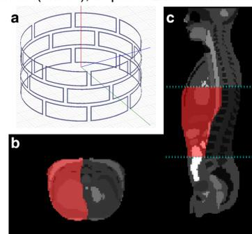
**Figure 1:** a) Z-stacked 3x8ch pTX coil configuration. b-c) Slices of model with corresponding target patterns (overlaid in red). b) central transversal slice. c) central sagittal slice.
