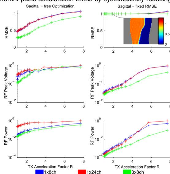
**Figure 2:** Simulation results of both optimization schemes (left free optimization, right fixed RMSE) for sagittal direction. 2D spatial selective RF pulse performance metrics for different coil configurations are noted as a function of TX acceleration factor R. Mind: RF power and RF voltage metrics have a logarithmic scale and were normalized to the overall maximum value. Exemplary a normalized flip angle map of the 3x8ch excitation for RMSE=1 is shown.
