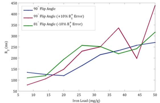
Figure 1 - Comparison of  $R_2$  values estimated from simulation runs showing that the ideal flip angle case produces lower  $R_2$  values than experiments with  $B_1^+$  inhomogeneity
