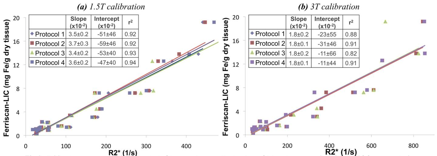
Fig 1: Calibration (mean ± standard error) of R2\* vs Ferriscan-LIC using four R2\* imaging protocols at 1.5T and 3.0T, respectively.
