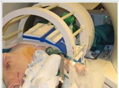
Fig. 3: Setup including the Tx birdcage and the Rx array on a 25 kg pig.
