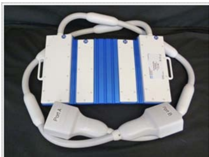
Fig. 2: The housing of the flexible Rx array has a total size of 23 x 40 cm 2 .
