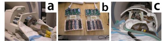
Figure 1. <sup>13</sup>C RF coils for human brain studies. a) transmit-receive birdcage volume coil, b) bi-lateral 8 channel <sup>13</sup>C receive coils, c) the set up showing the clamshell volumetric <sup>13</sup>C transmit coil and bi-lateral 8-channel phased array receive coils.
