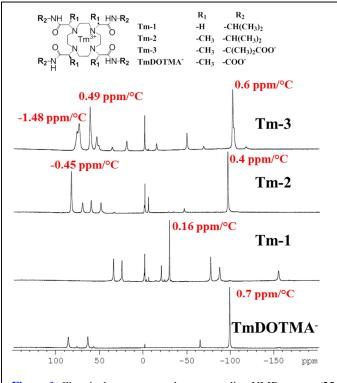
**Figure 1.** Chemical structures and corresponding NMR spectra (35 °C and pH 7.4) for the new BIRDS agents. Temperature sensitivities are indicated in red for the resonances of interest.
