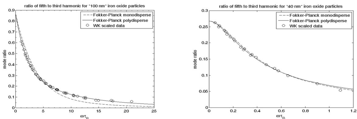
**Figure 1:** Measured and calculated ratio of the 5<sup>th</sup> to 3<sup>rd</sup> harmonics for the (a) “100 nm” and (b) “40 nm” iron oxide particles in glycerol-water ferrofluids. The measured values [3] (indicated by circles) are scaled as a function of  $\omega\tau_B$  (the drive frequency  $\omega$  times the Brownian relaxation time  $\tau_B$ .) The dashed (solid) line is the harmonic ratio from the FP approach with a monodisperse (polydisperse) model.
