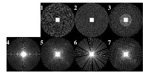
Fig. 3 k<sub>y</sub>-k<sub>z</sub> undersampling (R=6): 1) uniform random, 2) Poisson-Disk random, 3) variable-density Poisson-Disk random, 4) uniform radial, 5) golden-ratio radial, 6) randomized uniform radial, 7) randomized golden-ratio radial.
