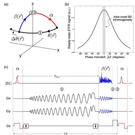
Figure 1: Small-tip fast recovery (STFR) imaging. (a) Steady-state spin path. The tip-up pulse (blue) is tailored to the local free precession angle  $\theta(r)=\omega(r)T_{free}$ . In general, there will be a mismatch  $\Delta\theta(r)$  between the tip-up phase and spin phase at end of the free precession interval. (b) Signal profile vs. phase mismatch. (c) STFR pulse sequence diagram, using a 2D spiral tip-up pulse and segmented 3D stack-of-spirals acquisition.
