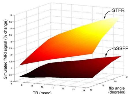
Figure 3: Monte Carlo Bloch simulation results: Percent functional signal change for STFR and bSSFP as a function of TR (7-14 ms) and flip angle ( $12^\circ$ - $24^\circ$  – the bSSFP flip angle is twice the value indicated). STFR fMRI is predicted to produce 3-5 fold signal increase relative to passband bSSFP.
