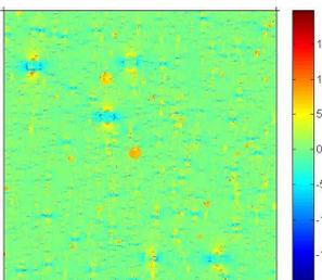
Figure 2: Microscopic B0 inhomogeneity (Hz) in the numerical voxel used in our Monte Carlo Bloch simulations. A 2D cut through the  $1 \times 1 \times 1 \text{ mm}^3$  voxel is shown.
