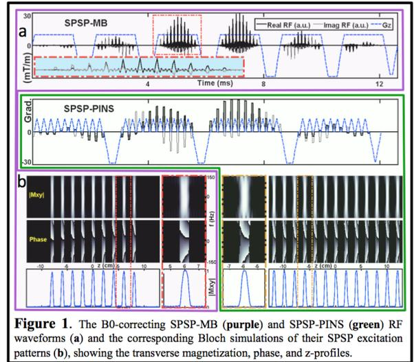
**Figure 1.** The B0-correcting SPSP-MB (purple) and SPSP-PINS (green) RF waveforms (a) and the corresponding Bloch simulations of their SPSP excitation patterns (b), showing the transverse magnetization, phase, and z-profiles.
