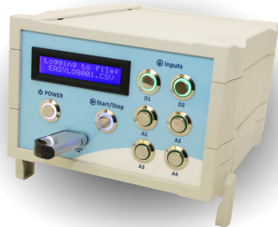
Figure 1: The stand-alone logging device is based on a microcontroller board Olimexino-STM32 with a 72 MHz clock. The board allows acquisition for up to 6 analog and 2 digital inputs. A front panel display shows the name of the currently logged file. Relatively small size (dimensions 17x13x20cm 3 , weight 1kg) of the device makes it easy to transport.
