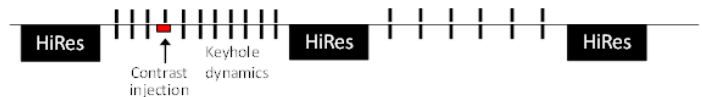
Fig 1. The DCE-MRI protocol. High spatial resolution acquisitions (90s) are acquired before contrast injection and at 2 min, 6.5 min after contrast injection. High temporal resolution acquisitions (15s/30s) are performed in between.
