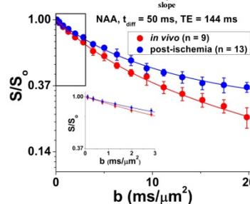
**Figure 1.** Semi-log plot of group-averaged NAA diffusion data for T<sub>NMR</sub> in the range from 36 – 38 °C. **Inset:** Fits of b < 3 ms/μm<sup>2</sup> data to S(b) = S<sub>0</sub> · e<sup>-b·ADC</sup> yield a pre-ischemia ADC for NAA of 0.122 ± 0.004 μm<sup>2</sup>/ms vs. 0.097 ± 0.003 μm<sup>2</sup>/ms post-ischemia, a 20% decrease.
