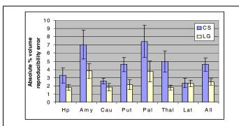
**Figure 1:** Across-session test-retest percent absolute volume reproducibility errors averaged across eight 3T MRI sites for the cross-sectional (CS) and longitudinal (LG) FreeSurfer segmentation streams.
