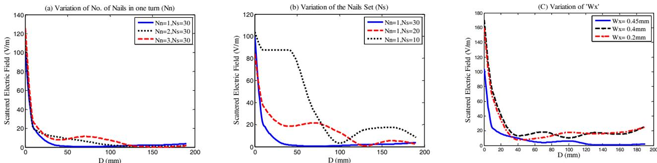
Fig. 4. Simulation results for variation of (a) No. of nails in one turn, Nn; (b) Nails set, Ns; (c) Nail length, Wx
