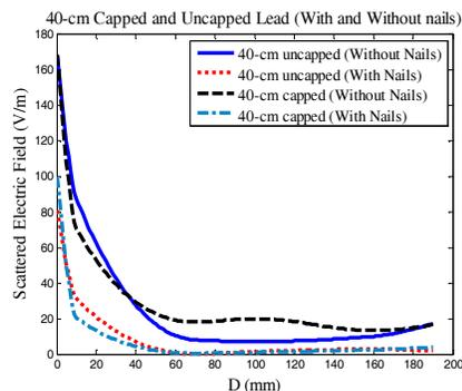
Fig. 3. Simulation results for with and without nails configuration of 40-cm capped and uncapped lead
