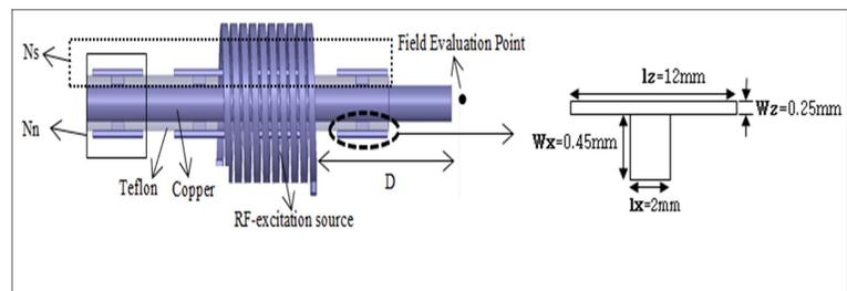
Fig. 2. Model of the medical lead Implant with proposed nails and RF source
