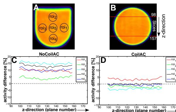
**Figure 2:** (A) Axial PET image shows the 5 circular ROIs used for quantitative evaluation of the local attenuation due to the RF coil. (B) Coronal PET image illustrates the range of reconstructed axial planes plotted in graphs (C) and (D). (C) PET data sets with no AC of the coil. (D) PET data sets with CT-based AC of the RF coil.
