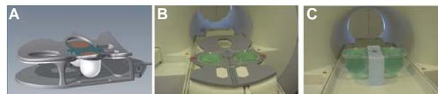
**Figure 1:** (A) Breast phantom positioned in the 4-Channel RF breast coil. (B) PET scan setup with RF breast coil and breast phantom. (C) PET scan setup with only the breast phantom as a reference scan.
