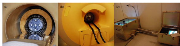
Fig. 1. The proposed MRI-PET system with a PET-insert. (a) Front and (b) rear views of the MRI-PET system, including the gantry and the RF coil. (c) A shield box to prevent RF noise from PET electronics.
