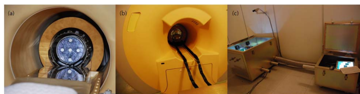
Fig. 1. The proposed simultaneous MRI-PET System with a PET-insert. (a) Front and (b) rear views of the MRI system after placing the PET gantry and the RF coil. (c) A shield box to prevent RF noise from PET electronics.
