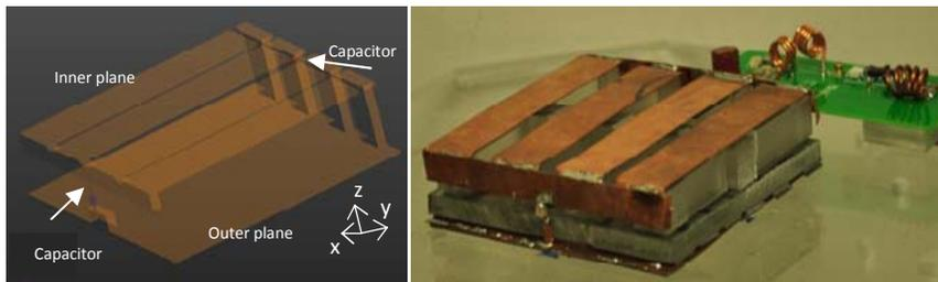
Fig. 1 A schematic of the bi-planar coil and the developed coil with a pre-amp circuit.
