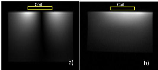
Fig. 3 Sagittal-view phantom images obtained with a) the square-loop coil and b) the bi-planar coil.
