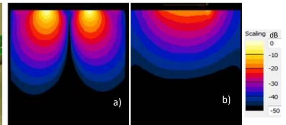
Fig.2 Simulated iso-contour plots of  $B_1$  magnitude for a) the square-loop coil and b) the bi-planar coil.
