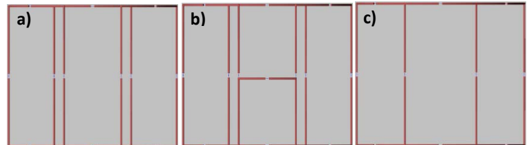
Fig. 1: The three different decoupling schemes: (a) overlapped array, (b) overlapped array with shared capacitor for next nearest neighbor decoupling, (c) shared conductor array.
