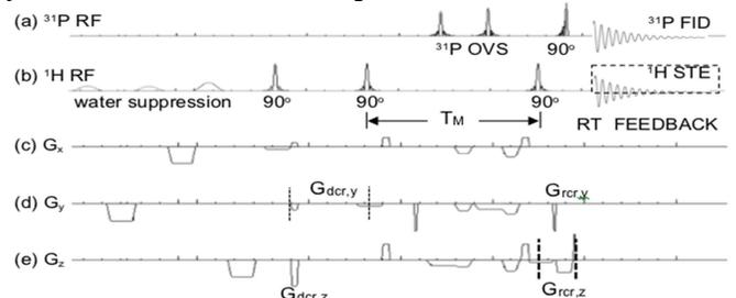
**Fig. 2.** Pulse sequence diagram for a simultaneous water suppressed  $^1\text{H}$  and  $^{31}\text{P}$  MRS: (a)  $^{31}\text{P}$  FID MRS using 2D-OVS + slice-selective excitation, (b) STEAM for  $^1\text{H}$  MRS with, (c - e) gradient waveforms. The dotted box indicates the data acquisition of the  $^1\text{H}$  signal.
