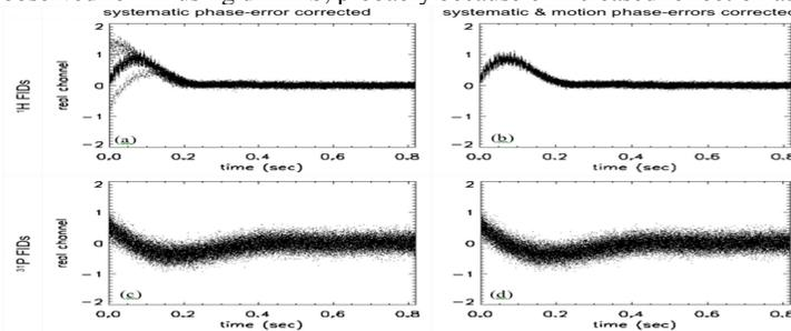
**Fig. 3.** 20 real-channel  $^1\text{H}$  FIDs are overlaid each other with (a) systematic phase-error correction and (b) systematic and motion-induced phase-error correction. Note negligible improvement in  $^{31}\text{P}$  FIDs, because the change in  $^{31}\text{P}$  phase is 40 % of that in  $^1\text{H}$  phase.
