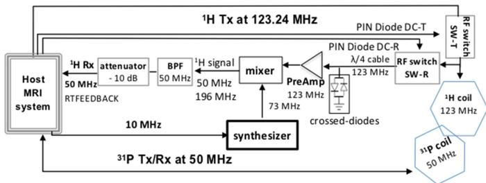
**Fig. 1.** Schematic block diagram for simultaneous dnMRS. Arrows indicate the directions of the Tx RF pulses and MR signals. The 123.23 MHz  $^1\text{H}$  signal is directed to  $^{31}\text{P}$  Rx pathway using two PIN-diode driven RF switches (SW-T and SW-R) and converted to 49.9 MHz.
