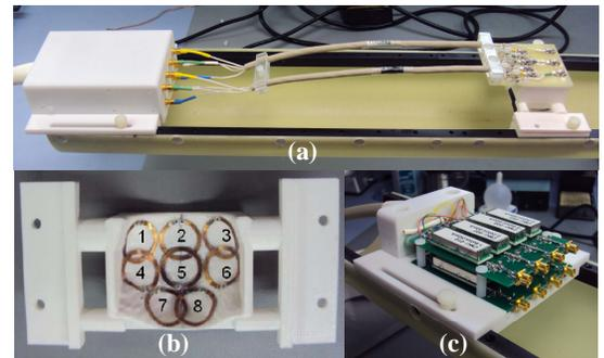
**Figure 1:** (a) 8-channel embedded array connected to low Z preamplifiers. (b) Bottom view of the arrangement of the individual array elements. (c) View of preamplifier set.
