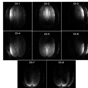
**Figure 4:** Shuffled images showing the spatial coverage of the 8-channel embedded array.
