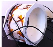
**Figure 1.** 8 channel receive only 6.5 mT parallel imaging array.
