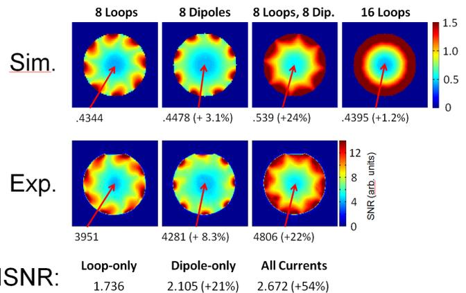
Figure 3: Optimum SNR maps, normalized for B<sub>1</sub><sup>+</sup> distribution, and values of Ultimate Intrinsic SNR for this geometry (arbitrary units).
