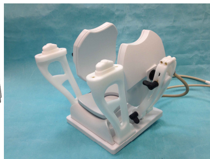
Fig. 2 Shows the realized coil, including provision for bite bar and mirror.
