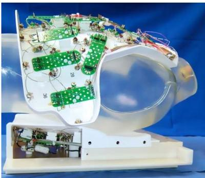
**Fig.4:** Implementation of the simulated 64-channel cardiac phased-array on chest and back
