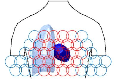
**Fig.1:** Final unwrapped coil configuration on the chest with diamond-shaped start pattern (red) and added coil elements on right/left side (blue) over the heart (dark blue)
