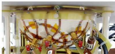
Figure 2. Photograph of custom designed housing with FCE coil with receive array insert.
