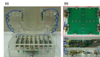
**Fig 1:** The (a) customized RF coil array consists of (b) dual four element RF coil arrays and (c) their RF circuitry.
