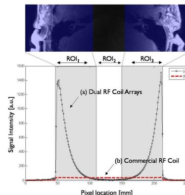
**Fig 2:** 2-D inner ear VIBE images from a healthy volunteer (upper part) and signal intensity profiles from a spherical phantom (bottom part). Signal intensity profiles for (a) RF coil arrays and (b) commercial RF BC volume coil through transverse slices passing approximately through the center of the spherical phantom.
