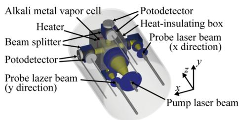
Fig. 1. Schematic of OPAM module for direct MR signal detection.
