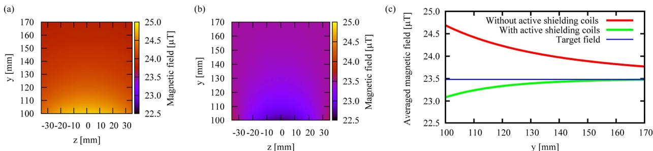
Fig. 3. The resulting magnetic field distributions in the vicinity of the sample without and with active magnetic shielded cancelling coils. (a) The magnetic field distribution with cancelling coil only. (b) The magnetic distribution with an active magnetic shielded cancelling coil. (c) The magnetic fields averaged along z direction in (a) and (b).
