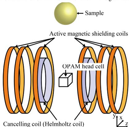
Fig.2. Schematic of an active magnetic shielded cancelling coils.
