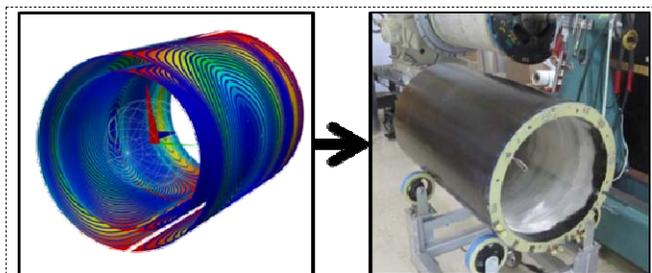
Figure 1: Pictures of the considered head gradient subsystem: from design to the first prototype.
