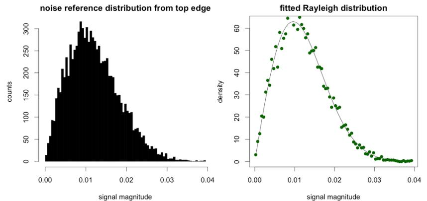
**Figure 1:** Empirical noise distribution (left) obtained by lumping all voxels along top edge of image at all 71 time points. The fit on the right is a Rayleigh distribution (solid black curve) with the original signal density overlaid in green.
