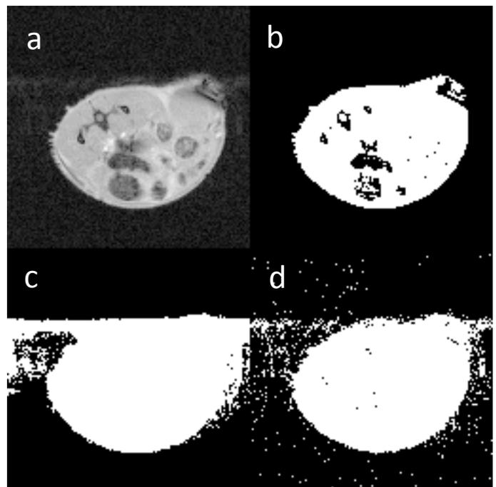
**Figure 2:** Square root of test image (a) and generated masks (b-d). Otsu's method missed areas of signal inside the mouse (b). Lowering the cutoff arbitrarily to 0.2 of the Otsu threshold captured more of the low-signal voxels, but incorrectly marked air voxels. The K-S test (c) found almost all signal, even the low-intensity aliased power, while ignoring noise outside the imaging volume.
