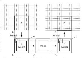
1.) Extraction of an overlapping block A 2.) Convolution with two applications of an FFT. The result is valid in region B (overlap-and-save). 3.) Multiplication of B with the sampling mask (in-place) and setting of the invalid part to zero. 4.) Adjoint convolution
