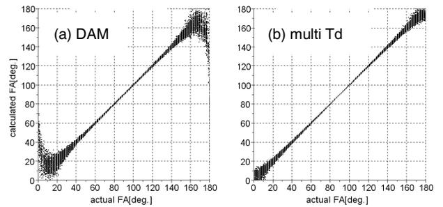
Fig. 2 Dynamic range of B<sub>1</sub> map (a) DAM, and (b) multi Td method
