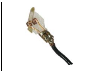
Figure 2: Home-built T/R field probe tuned at ^{19}\text{F} , and interfaced directly to the Philips MR system.
