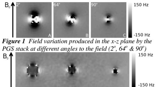
Figure 1 Field variation produced in the x-z plane by the PGS stack at different angles to the field ( $2^\circ$ ,  $64^\circ$  &  $90^\circ$ )
