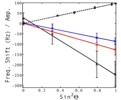
Figure 3 Variation with  $\sin^2 \Theta$  of internal field for 15, 10 & 5 mm diameter tubes (blue, red & black  $\times$ ; error bars = s.d.) and external field (black  $\circ$ ; bars = fit errors).
